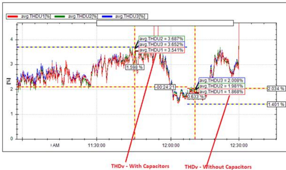
Fig 4 – Total Harmonic Distortion –V (THD-V) With and Without Capacitors
