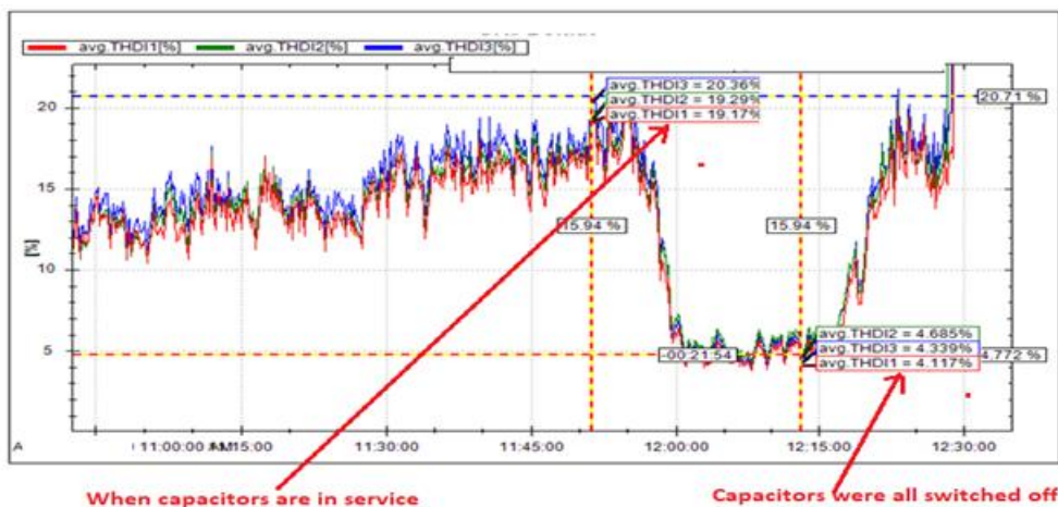
Fig 2 – Total Harmonic Distortion - Current (THD –I)
